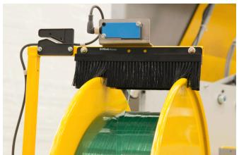
Auto strap feed and re-feed from dispenser into sealer for MHC heads.
