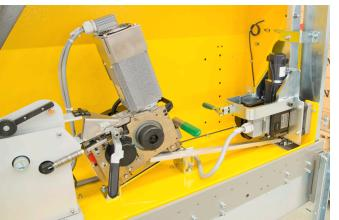
The easily accessible head carriage allows easy service work when needed. Signode MHC modular head technology improves performance and speed.
