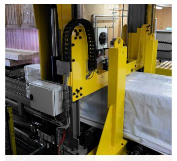
**Product protection** High speed but soft approach of the top and side compaction arms, reduces product surface damage.
