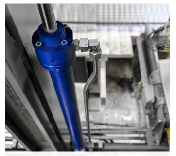
**Hydraulic compression drives** Fast, variable compression is quick and can be adjusted per product/pack being processed.
