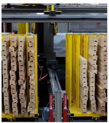
**Enhanced Productivity** Twin and up to quadruple batten magazines, each can be separately reloaded with no production stops.
