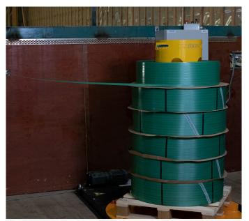
**Strap dispenser for coils up to 300kg.** From 70-300 kg coils of PET for more uptime, less coil changes plus much improved work safety.
