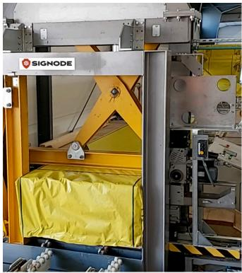
**Enhanced productivity** Side mounted Z20 head for easy strap loading and simpler service to be completed at floor level.
