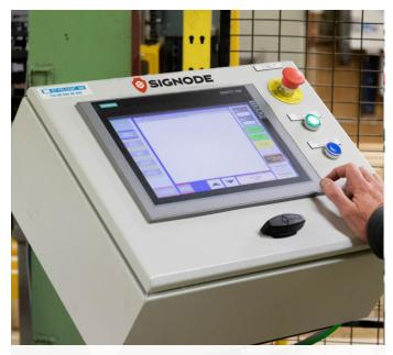
**Systems visualisation** Equipped with its own controller, it can be integrated into a complete line. (12" HMI shown is an option).
