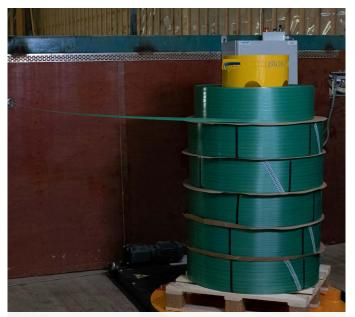
**Strap dispenser for coils up to 300kg.** From 70-300 kg coils of PET for more uptime and less coil changes.
