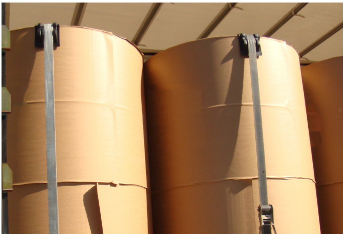
Jumbo corner applied to paper reels to protect against lashing abrasion.
