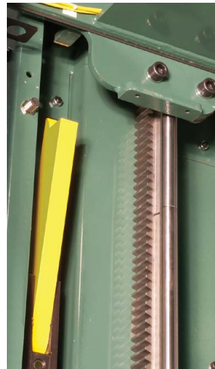
Auto latch conversion: Automatic platen latch activated and extended
