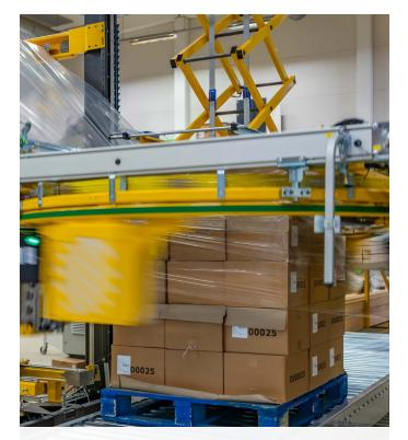
Real time data collection, on pallet during wrapping cycle
