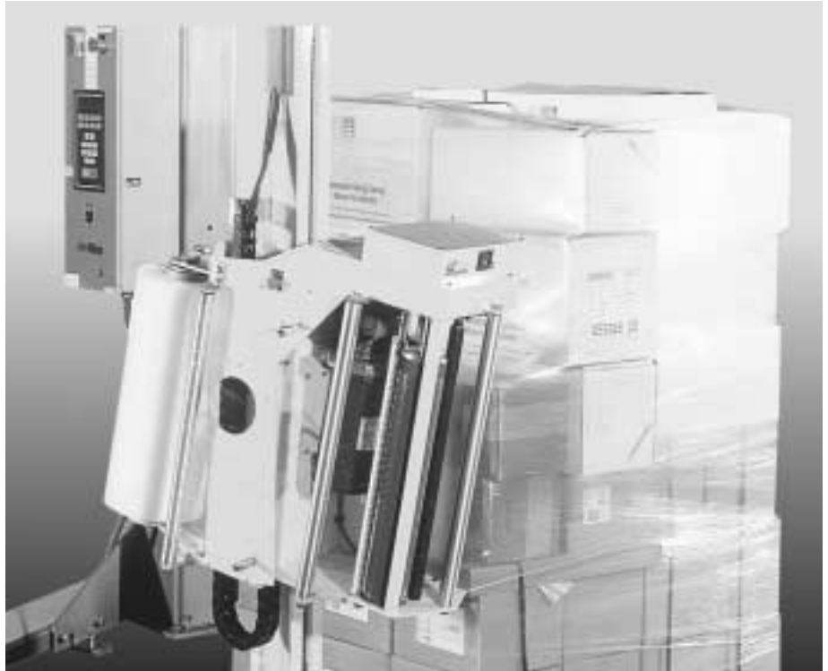
Manufactured with metallocene resins, Signode STO stretch film securely wraps even the toughest type C loads.
